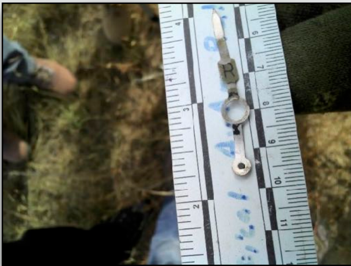
Needle from an engine manifold pressure gauge for either the left or right wing. (Photo Credit: Larry Liebrecht)
