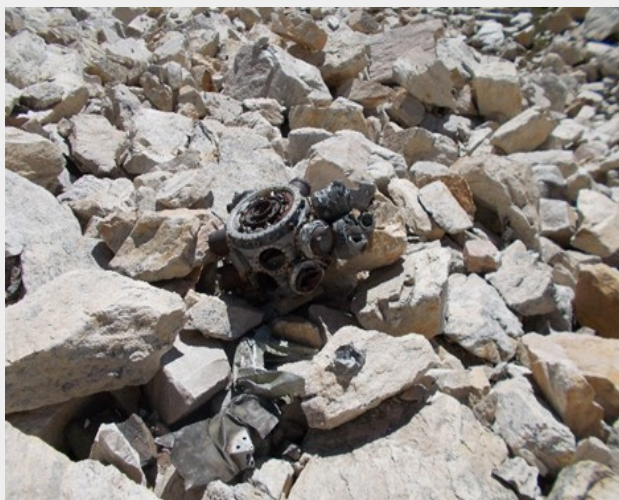
One of the P&W R-2000 engines near the bottom of the debris field (Photo: Brian Richardson)
