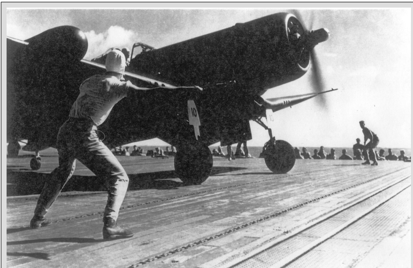
Brunson's aircraft #10 ready to roll. The AN/AP-4 Radome is visible on the starboard wing of this F4U-2 night fighter version of the Corsair. (Photo courtesy of Bob Brunson)
