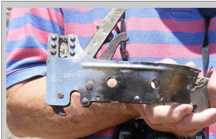
Mark Milliken displays a shackle used to suspend ordnance in the bomb-bay of the B-24. (photo: AvAr archives)
