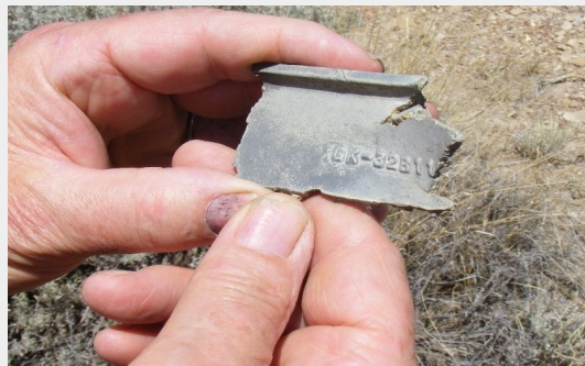
Proof of the aircraft's model/type: The 32 prefix of this part number indicates that this was a B-24 aircraft. (photo: AvAr archive)
