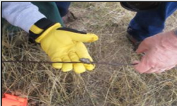
Confirmation: Length of barbed wire fence with melted aircraft aluminum attached.
