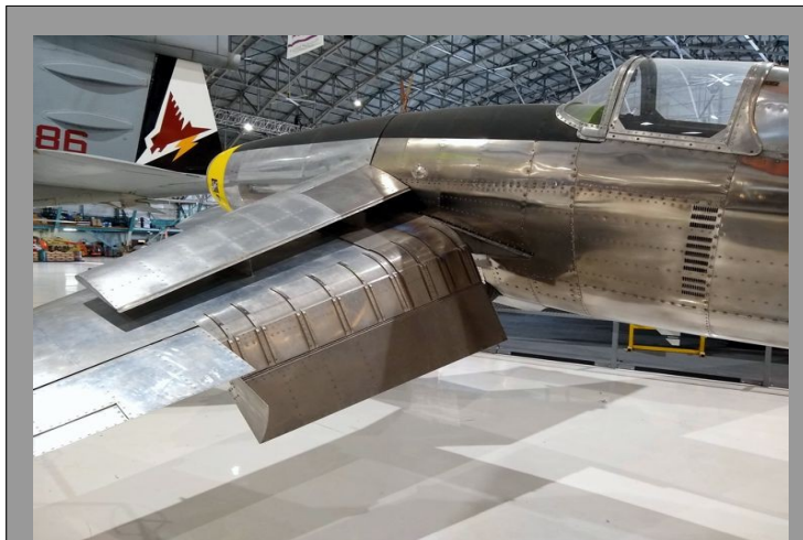
Detail of the "augmentor" wing and flaps on the Jetwing (photo: Jerry Thomas)
