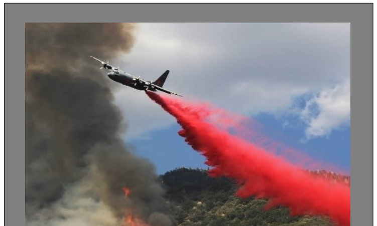
A 302 nd Airlift Wing MAFFS equipped C-130H (Modular Airborne Fire Fighting System) drops a load of fire retardant on a forest fire. The 302 nd AW is one of the Air Force Reserve units that provides this capability to the National Forest Service to fight forest fires around the country. (photo:USAF )
