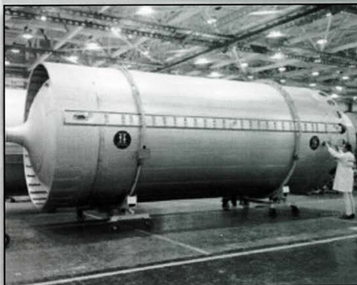
A Titan II fuel tank is inspected prior to shipment to the Baltimore Martin Company facility. (Lockheed/Martin Photo)
