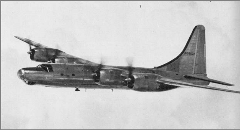
The TB-32 was the training version of the bomber. A total 116 of these aircraft were produced by Consolidated Aircraft. (Photo: General Dynamics)
