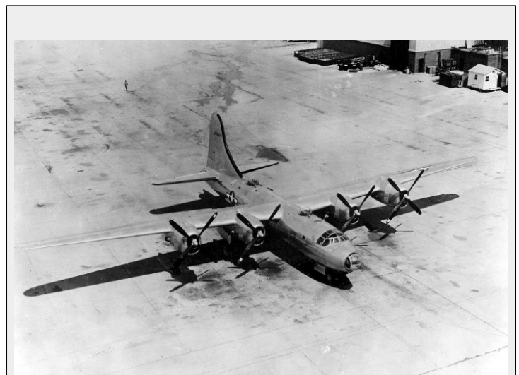
The consolidated B-32 was designed as a fall-back for the Boeing B-29. Only 116 were produced. (Photo: General Dynamics)
