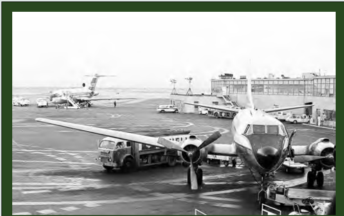
The Martin 404 was a twin-engine 40 passenger aircraft designed in the early 1950's as a replacement for the DC-3. Several local service airlines used this aircraft. (Photo: Steve Kelly)
