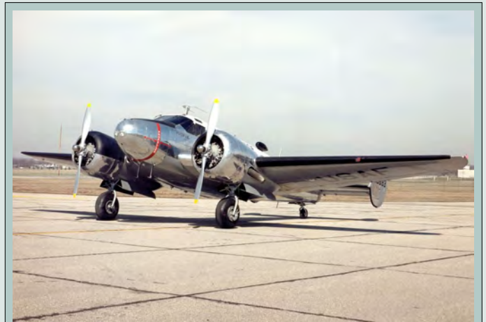
The C-45 was the military version of the popular Beech 18 model. (Photo: USAF Museum)
